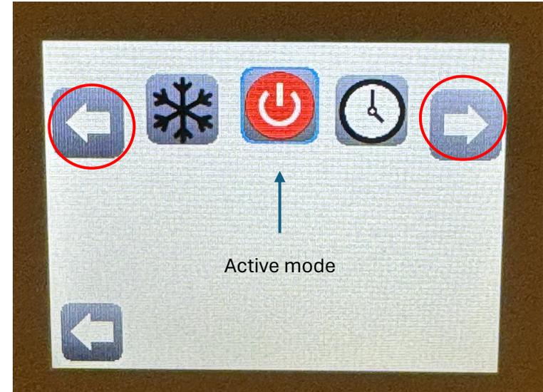
3. The modes menu is displayed. The highlighted white arrows let you scroll through a range of operational modes. The current active mode is framed in blue (in this case the 'Off' mode)
