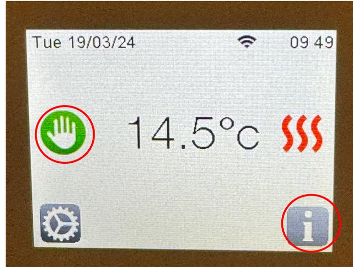
5. The manual mode screen appears (shown by the highlighted hand symbol). The current room temperature is displayed, and the 3 red wavy lines show that the room heating panels are on. These may take a few seconds to appear. If you want to set a different target temperature whilst in manual mode, touch the 'i' symbol on the bottom right.
