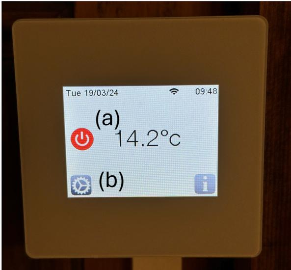
1. Room thermostat is in 'Off' mode when red power button (a) is visible. To turn on the room heaters, touch the 'cog' symbol (b)
