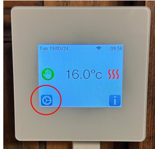
8. To turn the room heaters off, touch the cog symbol at the bottom left (highlighted in red).
