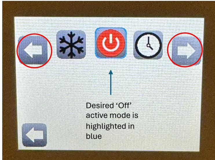
10. Use the white arrows (highlighted) to scroll through the operational modes until 'Off' mode is framed in blue. Then touch the back arrow at the bottom left to make 'Off' the active mode.
