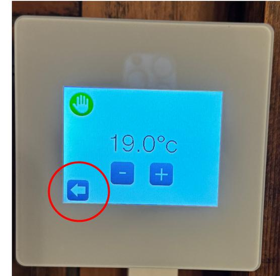
6. The manual temperature adjust screen is displayed. Alter the desired target temperature as required using the + and - buttons and then click the white arrow on the bottom right.
